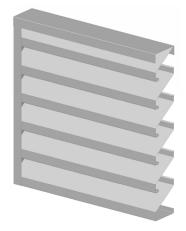
Kovach's Metal Louvers allow very little water penetration while maintaining airflow. Designed with jam gutters, our louvers are drainable and direct water out and away from the opening. Mill finish, standard and custom colors are available in a fluoropolymer (Kynar) painted finish. Louvers provided by Kovach include shop drawings specific to each project.
